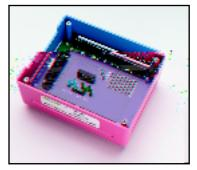
**STA-08PGA:** The STA-08PGA provides one 37-pin Dtype male connector for hook up to the DAS-801 and DAS-802. All signals are routed to labeled screw terminal connections. The digital I/O lines are connected to 7 LEDs to indicate their status. A small breadboard area with power is provided.
