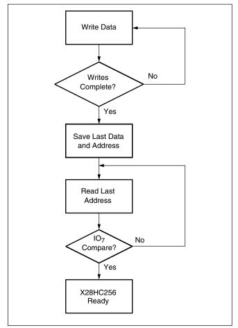
DATA Polling can effectively halve the time for writing to the X28HC256. The timing diagram in Figure 2 illustrates the sequence of events on the bus. The software flow diagram in Figure 3 illustrates one method of implementing the routine.
