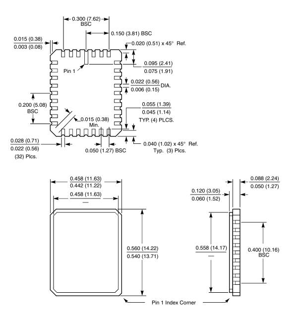
NOTE: 1. ALL DIMENSIONS IN INCHES (IN PARENTHESES IN MILLIMETERS) 2. TOLERANCE: ±1% NLT ±0.005 (0.127)
