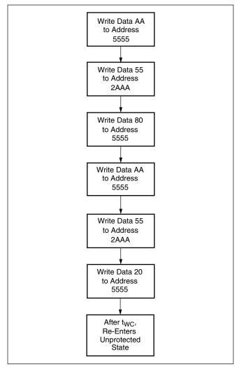
In the event the user wants to deactivate the software data protection feature for testing or reprogramming in an EEPROM programmer, the following six step algorithm will reset the internal protection circuit. After  $t_{WC}$ , the X28HC256 will be in standard operating mode.
