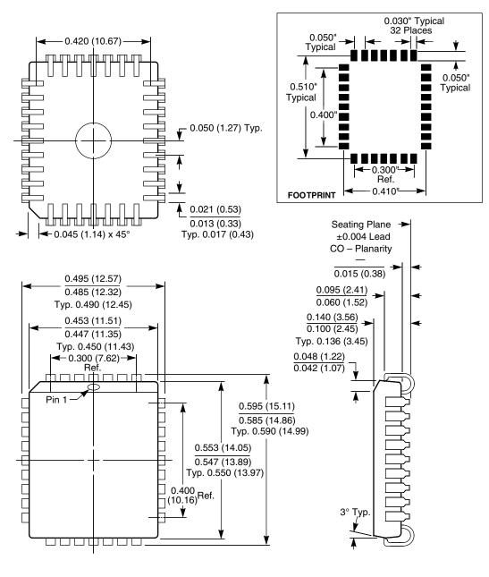
NOTES: 1. ALL DIMENSIONS IN INCHES (IN PARENTHESES IN MILLIMETERS) 2. DIMENSIONS WITH NO TOLERANCE FOR REFERENCE ONLY
