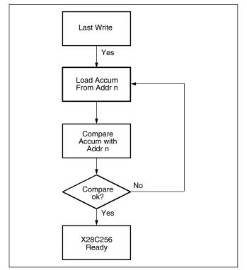
The Toggle Bit can eliminate the chore of saving and fetching the last address and data in order to implement DATA Polling. This can be especially helpful in an array comprised of multiple X28HC256 memories that is frequently updated. The timing diagram in Figure 4 illustrates the sequence of events on the bus. The software flow diagram in Figure 5 illustrates a method for polling the Toggle Bit.
