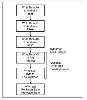
Regardless of whether the device has previously been protected or not, once the software data protection algorithm is used and data has been written, the X28HC256 will automatically disable further writes unless another command is issued to cancel it. If no further commands are issued the X28HC256 will be write protected during power-down and after any subsequent power-up.
