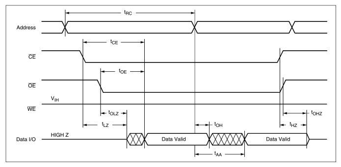
Notes: (4) t<sub>LZ</sub> min., t<sub>HZ</sub>, t<sub>OLZ</sub> min. and t<sub>OHZ</sub> are periodically sampled and not 100% tested, t<sub>HZ</sub> and t<sub>OHZ</sub> are measured with CL = 5pF, from the point when CE, OE return HIGH (whichever occurs first) to the time when the outputs are no longer driven.
