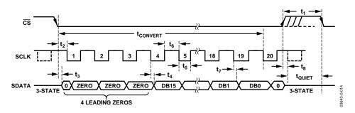
Figure 21. AD7680 Serial Interface Timing Diagram—20 SCLK Transfer
