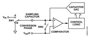
Figure 12. ADC Conversion Phase
