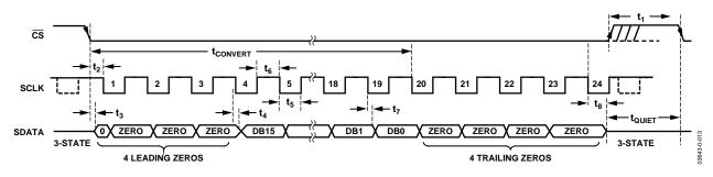
Figure 20. AD7680 Serial Interface Timing Diagram—24 SCLK Transfer
