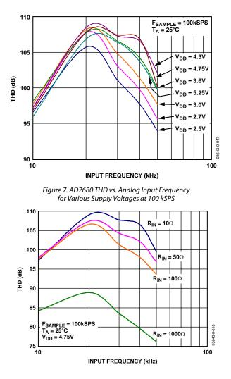
Figure 8. AD7680 THD vs. Analog Input Frequency for Various Source Impedances
