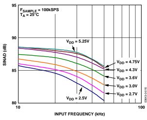
Figure 6. AD7680 SINAD vs. Analog Input Frequency for Various Supply Voltages at 100 kSPS
