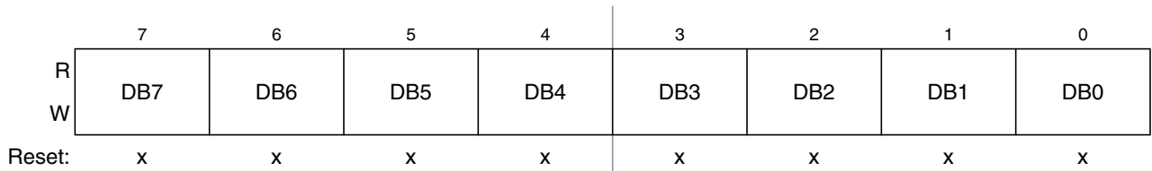
Figure 10-32. Data Segment Registers (DSR0–DSR7) — Extended Identifier Mapping
