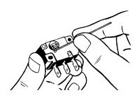
Push the lever down in the direction of the groove in the rotary disc.
