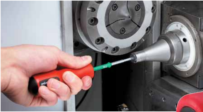
With the easyTorque, assembling indexable inserts is safe and easy.
