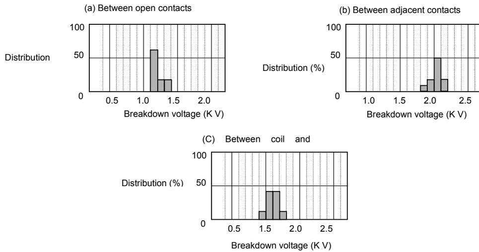
□ ALTERNATION OF VOLTAGE IN DENSE MOUNTING (magnet interference)
