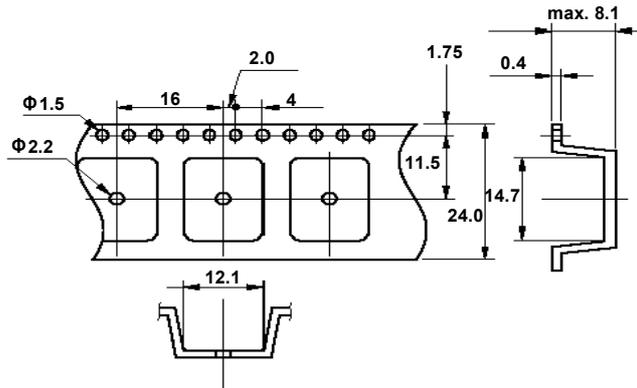
RELAY DIRECTION MARK AND TAPE CARRYING DIRECTION
