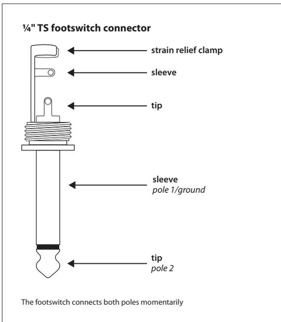
Fig. 4.1: 1/4" TS connector for foot switch
