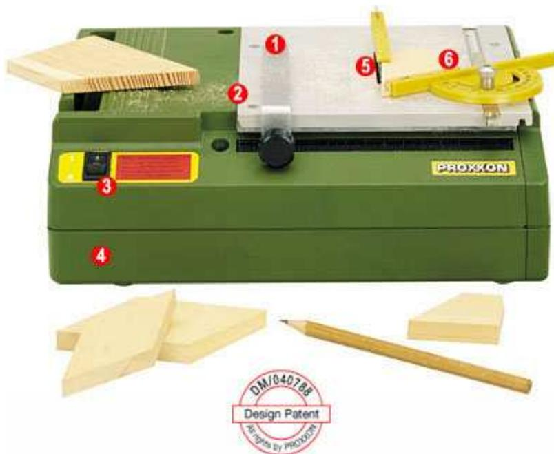
The 58mm diameter super-cut blade cuts soft woods up to 8mm. The 85W VDE tested motor is quiet, operates off 220 - 240V and has a prolonged life expectancy. Cutting performance: in wood up to 8mm, plastics (Pertinax too) to approx. 3mm, non-ferrous metals to approx. 1.5mm. Even fibreglass reinforced PC cards can be cut with the tungsten blade. The side door allows easy sawdust removal. Overall size approx. 240 x 180 x 80mm. Weight approx. 1.8kg.
