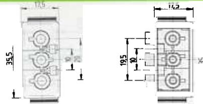
For fast mounting of female/male plug connectors, e. g. in cases of lighting devices or in plug boxes the snap-in version can be interlocked without using screws. The case opening is cleanly covered.
