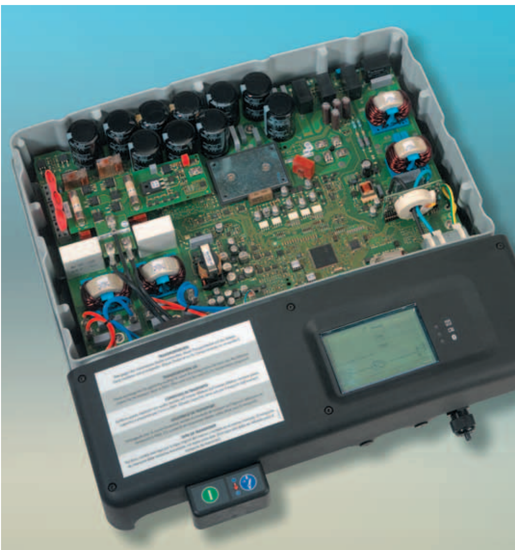
Figure 4: Modern 5 kWp inverter from SMA with relays from Tyco Electronics (top left RP relay and top right PCFN Solar)
