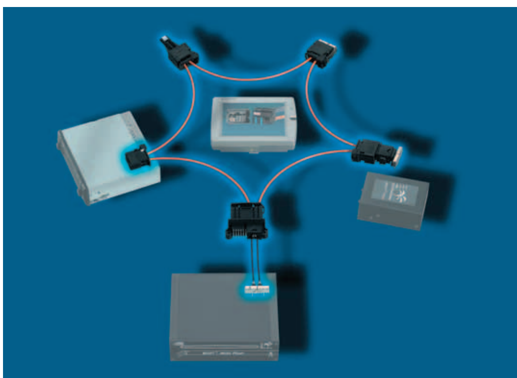
Picture 1: Example of MOST Network
