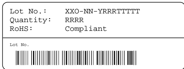
Figure 13: First label on reel: XX = Sensor Type (21 for SHT21), O = Output mode (D = Digital, P = PWM, S = SDM), NN = Chip Version, Y = last digit of year, RRR = number of sensors on reel divided by 10 (200 for 2000 units), TTTTT = Traceability Code.
