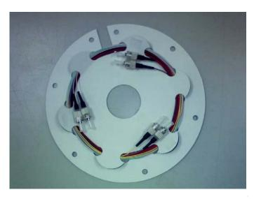
These coloured pigtails complement the use of colour coded fibre in loose tube cables. Usually 12 different coloures are used in either IEC or Bellcore coding. These pigtails use the same 12 colours, thus can be used for applications with both colour codes. The use of these colour coded pigtails makes the termination of fibre cable in patch panels or termination terminals easier and safer. Due to clear dedications, the risk of wrong fibre connections is reduced.
