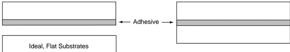
In this case, thermal impedance of the bond area,  $R_{tot}$  ( $^{\circ}\text{C}/\text{W}$ ), would be equal to the adhesive thermal resistance ( $^{\circ}\text{C}/\text{in}^2/\text{W}$ ) divided by the bond area,  $A_{tot}$  ( $\text{in}^2$ ). (Thermal resistance values typical of the 3M™ Thermally Conductive Tapes can be found in the Data Page.) To optimize thermal performance one would simply use the thinnest adhesive available.
