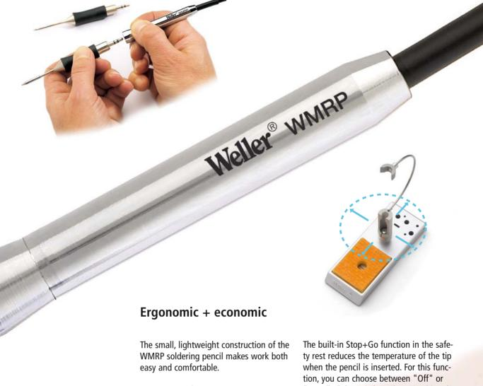
The WMRH safety rest has been designed with the latest ergonomic considerations in mind. Though it may appear unusual at first glance, the special geometry of the holder actually relieves the wrist of a substantial amount of strain. It avoids the usual turning and tilting motions, giving the user's wrist a break. The holder can be adjusted individually with a ball-and-socket joint at the base.
