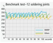
The WMRP soldering pencil has an extremely short heat-up time.\* (Approx. 2 seconds from standby to setpoint temperature!) All component parts of the system, such as the sensor and heating element, are designed for optimum heat transfer. This ensures absolute efficiency in the utilization of the power provided by the supply unit.
