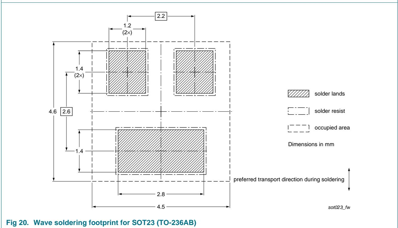
Fig 20. Wave soldering footprint for SOT23 (TO-236AB)
