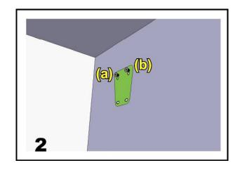
Slightly fasten the screws to (a) and (b) as indicated, and make sure the screws are not fully tightened.
