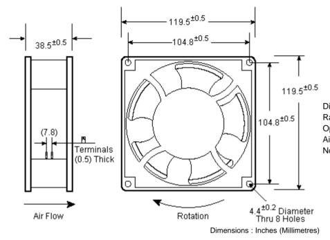
Dimension : 120 x 120 x 38mm. : 220V ac 50/60 Hz. Rated voltage Operating voltage Air flow Noise level
