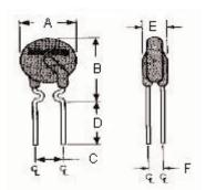
Lead Size : 24 AWG Ø0.51 mm Diameter
