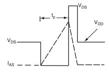
Fig. 12b - Unclamped Inductive Waveforms
