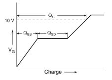
Fig. 13a - Basic Gate Charge Waveform
