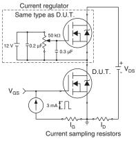
Fig. 13b - Gate Charge Test Circuit
