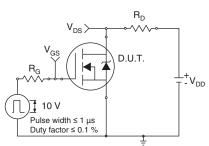
Fig. 10a - Switching Time Test Circuit
