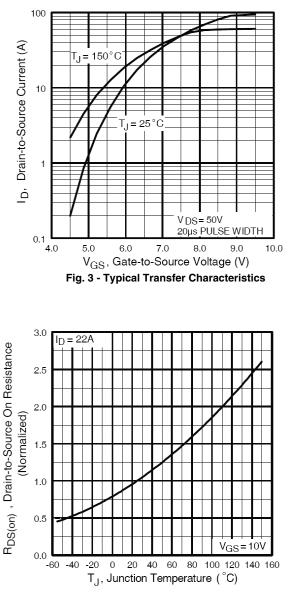
Fig. 4 - Normalized On-Resistance vs. Temperature
