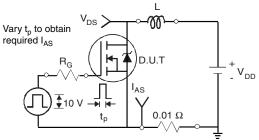
Fig. 12a - Unclamped Inductive Test Circuit
