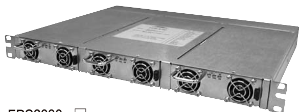
FPS3000 - □ Shelf type: 3 units of FPS1000 mounting in a 19-inch shelf (FPS-S1U) with maximum 3kW Size: 440(W)×43.6(H)×351(D) mm
