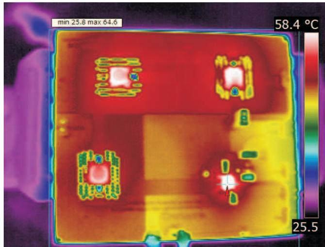
Figure 6. TL4242EVM-543 Top Infrared at  $V_{in} = 12\text{ V}$ ,  $I_{LED} = 357\text{ mA}$  (Viewed From Top)
