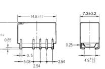
Footprint (Bottom View) Tolerance:  $\pm 0.1$ 2.54100 Ten, 1-dia. holes  $5.08\pm0.1$ (1.05)5.082.542.542.542.542.542.542.542.542.542.54
