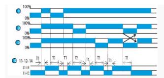
EWS/EWS2 relays monitor the correct sequencing of phases L1, L2 and L3 as well as the loss of one of these phases. When the phase sequence is correct, the output relay is energised, indicated by a yellow LED.
