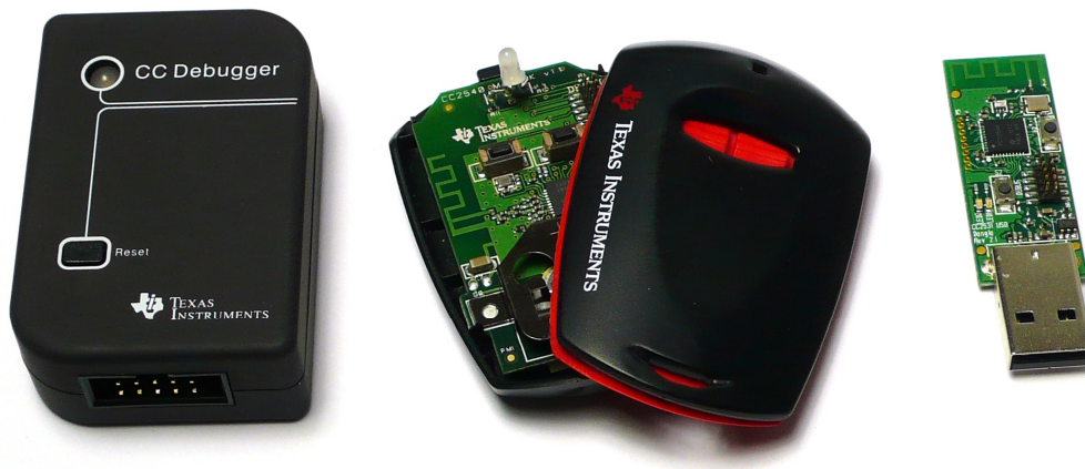
Figure 1 – Hardware Included with CC2540DK-MINI
