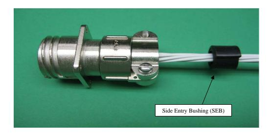
6. Slide the bushing forward and center it under the clamping bracket.
