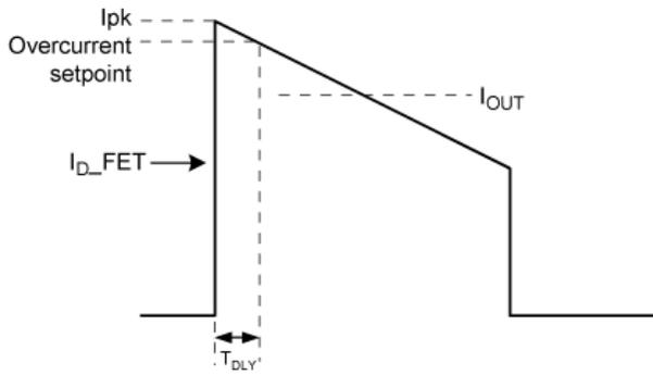
**Figure 9. Overcurrent waveform**
