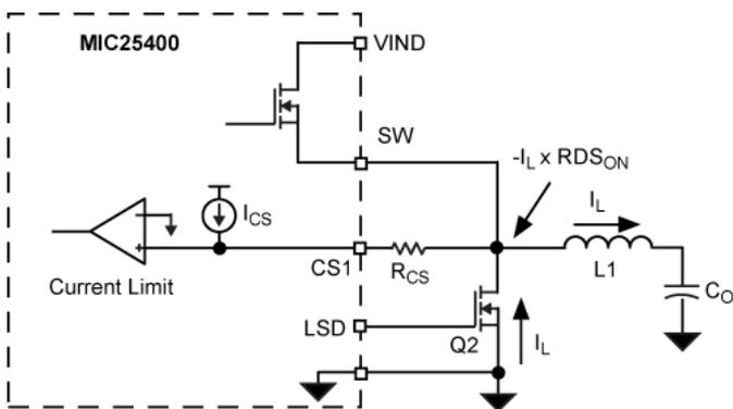
Figure 7. Over-current Circuit
