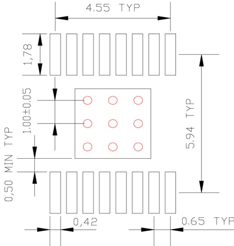
Red circle indicates Thermal Via. Size should be .300-.350 mm in diameter and it should be connected to GND plane for maximum thermal performance.
