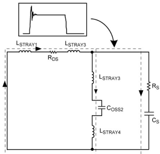
**Figure 11. Snubber Circuit**
