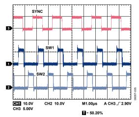
Figure 35. External Synchronization with 60° Phase Shift
