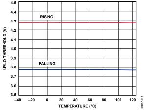
Figure 11. UVLO Threshold vs. Temperature
