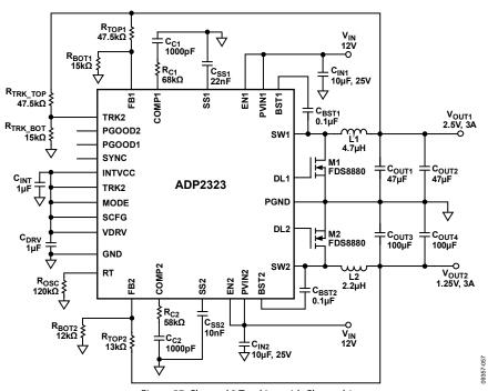
Figure 57. Channel 2 Tracking with Channel 1  $V_{IN1} = V_{IN2} = 12 \text{ V}$ ,  $V_{OUT1} = 2.5 \text{ V}$ ,  $I_{OUT1} = 3 \text{ A}$ ,  $V_{OUT2} = 1.25 \text{ V}$ ,  $I_{OUT2} = 3 \text{ A}$ ,  $f_{SW} = 500 \text{ kHz}$
