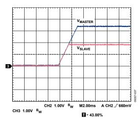
Figure 37. Coincident Tracking
