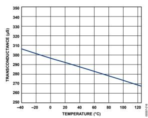
Figure 16.  $g_m$  vs. Temperature
