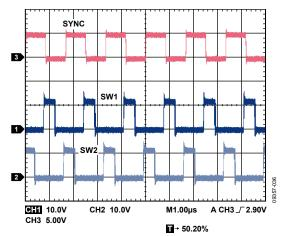
Figure 36. External Synchronization with 120° Phase Shift
