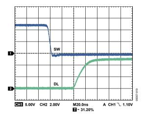
Figure 19. Low-Side Driver Rising Edge Waveform,  $C_{DL} = 2.2 \text{ nF}$
