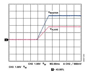
Figure 40. Ratiometric Tracking
