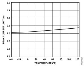
Figure 26. Current-Limit Threshold vs. Temperature,  $R_{\text{ILIM}} = 47 \text{ k}\Omega$
