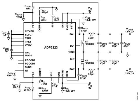
Figure 55. Enable PFM Mode with MODE Pin Pulled to GND,  $V_{IN1} = V_{IN2} = 9 V$ ,  $V_{OUT1} = 1.5 V$ ,  $I_{OUT1} = 3 A$ ,  $V_{OUT2} = 2.5 V$ ,  $I_{OUT2} = 3 A$ ,  $I_{SW} = 600 \text{ kHz}$
