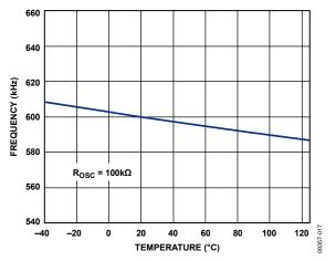
Figure 17. Frequency vs. Temperature
