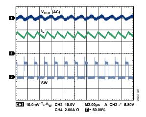
Figure 27. Continuous Conduction Mode (CCM)
