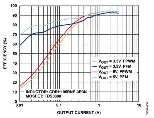
Figure 6. Efficiency at  $V_{IN} = 12 V$ ,  $f_{SW} = 600 kHz$ , PFM
