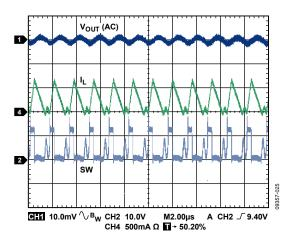
Figure 25. Discontinuous Conduction Mode (DCM)
