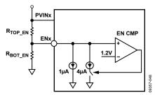
Figure 46. Programming UVLO Input
