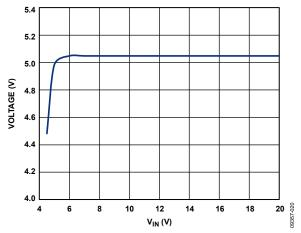
Figure 20. INTVCC Voltage vs. V<sub>IN</sub>
