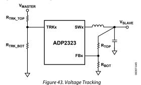
A common application is coincident tracking, which is shown in Figure 44. Coincident tracking limits the slave output voltage to be the same as the master voltage until it reaches regulation. For coincident tracking, set  $R_{TRK\_TOP} = R_{TOP}$  and  $R_{TRK\_BOT} = R_{BOT}$ .
