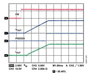
Figure 29. Soft Start With Full Load
