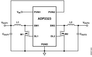
Figure 41. Cascading Supply Operation
