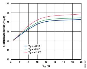
Figure 7. Shutdown Current vs. VIN
