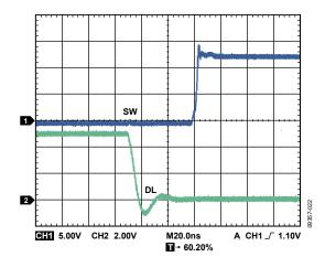
Figure 22. Low-Side Driver Falling Edge Waveform,  $C_{DL} = 2.2 \text{ nF}$
