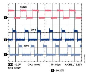
Figure 38. External Synchronization with 90° Phase Shift
