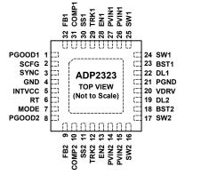
NOTES 1. THE EXPOSED PAD SHOULD BE SOLDERED TO AN EXTERNAL GND PLANE.
