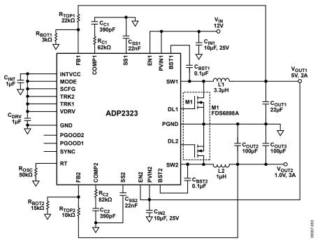
Figure 53. Cascading Supply Application,  $V_{IN1} = 12 \text{ V}$ ,  $V_{OUT1} = 5 \text{ V}$ ,  $I_{OUT2} = 2 \text{ A}$ ,  $V_{OUT2} = 1 \text{ V}$ ,  $I_{OUT2} = 3 \text{ A}$ ,  $f_{SW} = 1.2 \text{ MHz}$
