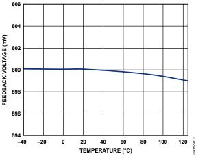
Figure 13. FB Voltage vs. Temperature
