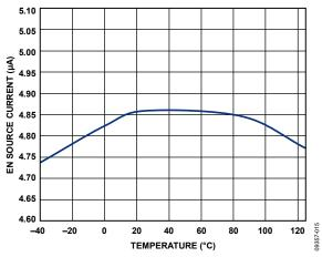
Figure 15. EN Source Current at  $V_{EN} = 1 V$
