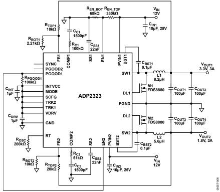
Figure 56. Programmable  $V_{IN\_RISING} = 8.7 \text{ V, } V_{IN\_FALLING} = 6.7 \text{ V, } 3.3 \text{ V Start Up Before } 1.8 \text{ V, } V_{IN1} = V_{IN2} = 12 \text{ V, } V_{OUT1} = 3.3 \text{ V, } I_{OUT1} = 3 \text{ A, } V_{OUT2} = 1.8 \text{ V, } I_{OUT2} = 3 \text{ A, } f_{SW} = 300 \text{ kHz}$
