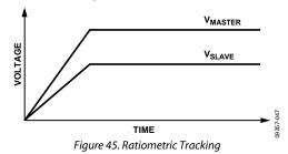
The ratio of the slave output voltage to the master voltage is a function of the two dividers, as follows:
