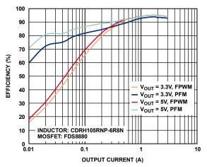
Figure 9. Efficiency at  $V_{IN} = 12 V$ ,  $f_{SW} = 300 kHz$ , PFM
