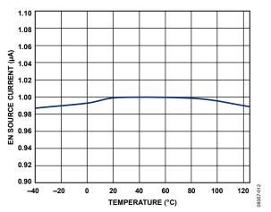
Figure 12. EN Source Current at  $V_{EN} = 1.5 \text{ V}$
