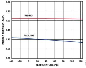
Figure 14. EN Threshold vs. Temperature
