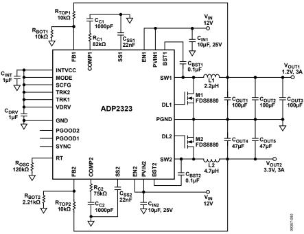
$Figure 50. \ Using \ External \ MOSFET \ Application, \ V_{IN1} = V_{IN2} = 12 \ V, \ V_{OUT1} = 1.2 \ V, \ I_{OUT1} = 3 \ A, \ V_{OUT2} = 3.3 \ V, \ I_{OUT2} = 3 \ A, \ f_{SW} = 500 \ kHz$
