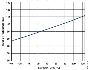
Figure 18. MOSFET R<sub>DSON</sub> vs. Temperature
