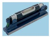
Precision ground base with full vee for location on cylindrical work pieces. Both levels have a main vial with safety cover, also a cross vial and a plumb vial. Main vial is graduated. All vials filled with tinted liquid for easy reading. Sensitivity - 1 minute of arc.
