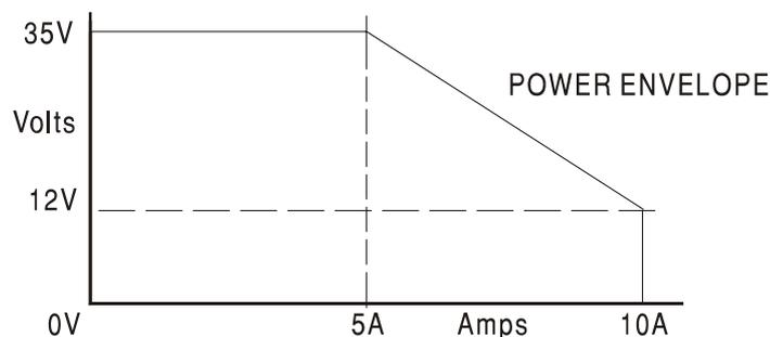
The power envelope is set to give 35V/5A and 12V/10A under all supply conditions (both outputs loaded); at lower output voltages the output power is restricted by the 10A current maximum.
