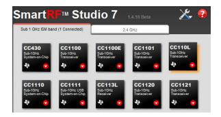
After installing the tool, connect the EB to the PC using the USB cable and start SmartRF Studio. Select the "Sub 1 GHz" tab and double click the highlighted device icon (CC110L, CC113L or CC115L).
