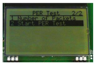
When selecting "Start PER Test", the master Press the "Up" button to go to the detailed (receiver) will begin to count the number of statistical window. received packets and provide some statistics.
