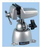
A very high quality, bench mounting vice which is fully adjustable with tilt, turn and swivel around the advanced ball and socket mechanism which supports the jaws. The jaws are adjusted with a wheel mechanism; ideal for fast, yet precise, adjustment. The jaws have a capacity from  $0\pm70$ mm and have nylon jaws to prevent damage to irregularly shaped objects
