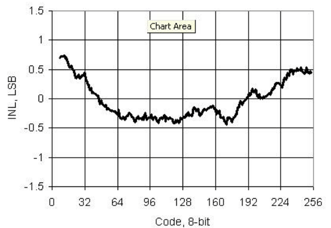
Figure 11-40. IDAC INL vs Input Code, Range = 255 \mu A, Sink Mode
