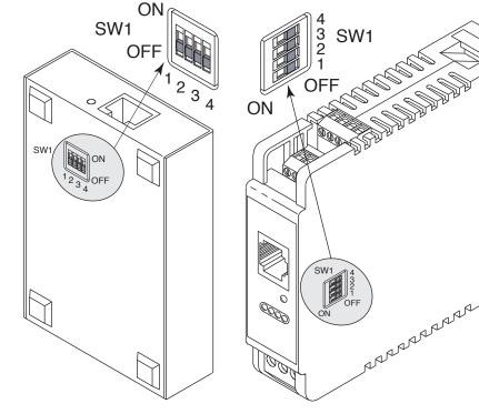
Figure 2.4a DIP Switch Wall Mount iServer
