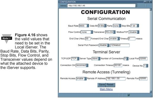
Figure 4.16 Local iServer (Serial-to-Ethernet model) Configuration Page
