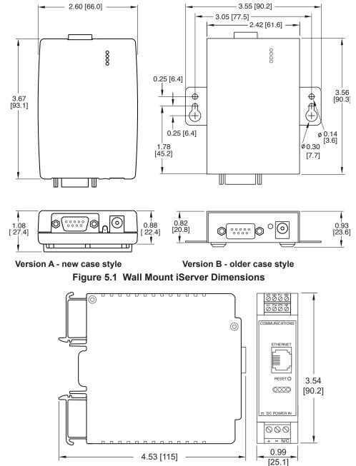
Figure 5.2 DIN Rail iServer Dimensions
