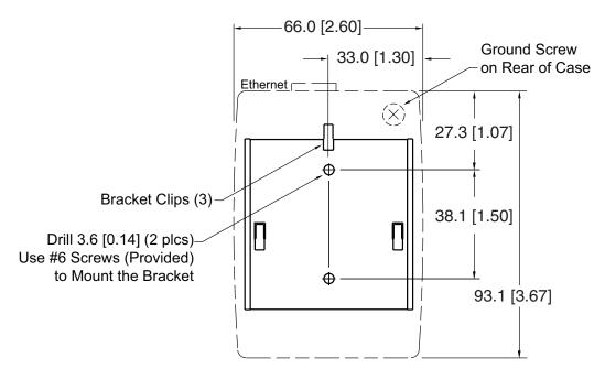
Figure 2.1 Mounting - Wall Mount iServer
