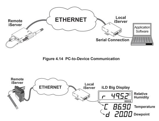
Figure 4.15 Device-to-Device Communication
