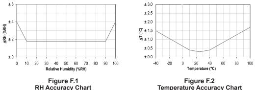
Accuracies are tested at Manufacture's Outgoing Quality Control at 25°C (77°F) and 3.3V. Values exclude hysteresis and non-linearity, and is only applicable to noncondensing environments.
