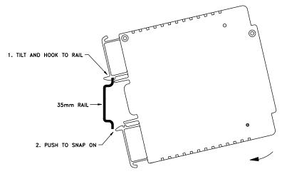
Figure 2.2 Mounting - DIN Rail iServer
