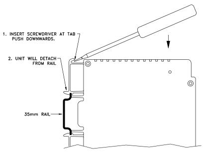
Figure 2.3 Removal - DIN Rail iServer
