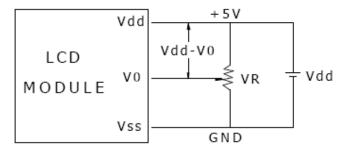
Vdd-V0: LCD Driving Voltage
