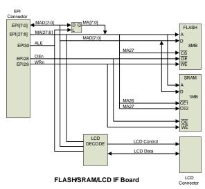
The Flash and SRAM memory expansion board has the following features:
