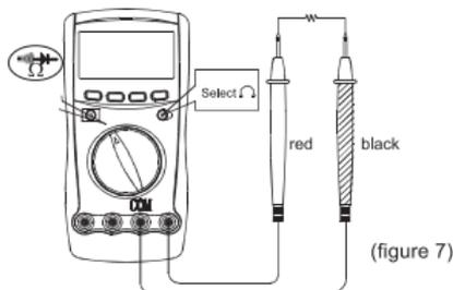
The resistance ranges are: 400.0 $\Omega$ , 4.000k $\Omega$ , 40.00k $\Omega$ , 400.0k $\Omega$ , 4.000M $\Omega$  and 40.00M $\Omega$ . To measure resistance, connect the Meter as follows:
