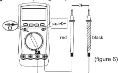
Use the diode test to check diodes, transistors, and other semiconductor devices. The diode test sends a current through the semiconductor junction, and then measures the voltage drop across the junction. A good silicon junction drops between 0.5V and 0.8V.
