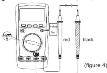
The DC Voltage ranges are: 400.0mV, 4.000V, 40.00V, 400.0V and 1000V. To measure DC voltage, connect the Meter as follows:
