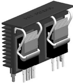
Ohmite introduces the C series (Pat. Pending). This series offers high performance, low cost and a compact heat sink with an integrated camming clip system for TO-247 packages (TO-220 and TO-264 available). This powerful heat sink provides tool and fixture free assembly operation, largest surface areas and smallest space occupation. It is the ideal type of heat sink for high power density and small size (1U or 2U) electronic packaging with forced convection cooling.
