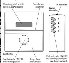
General The RLS010 is a standard size replacement wall switch for dimming filament lamps only up to 300W. The light under control can either be switched ON or OFF by a brief press of the push button on the switch itself or on the remote controller.
