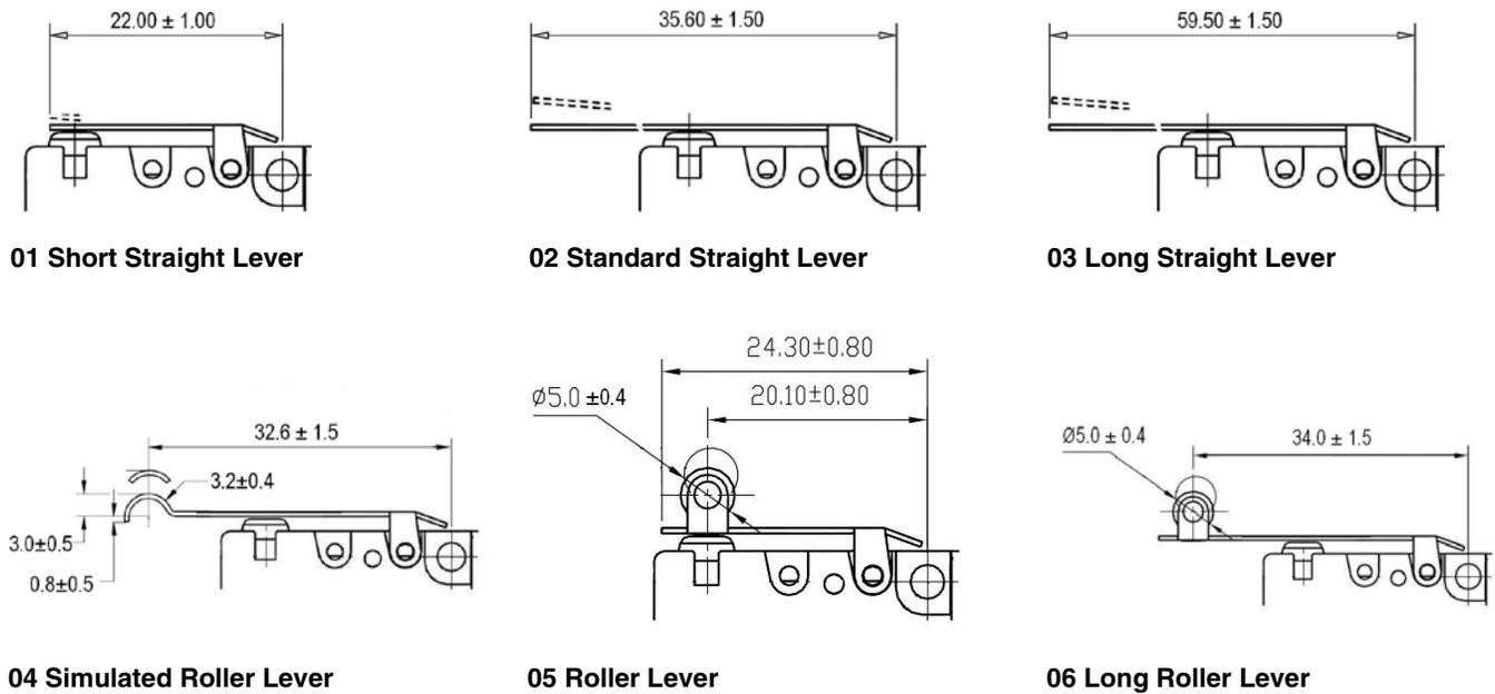
Figure 5. MICRO SWITCH™ V15W Series Watertight Miniature Basic Switch Operating Characteristics
