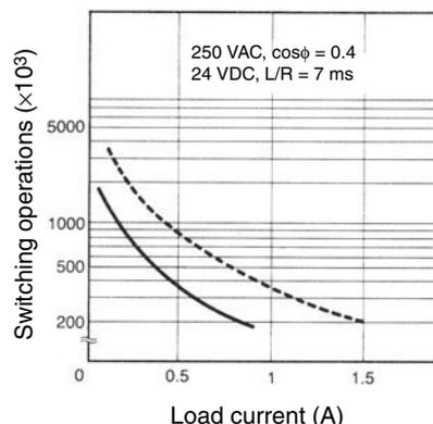
Reference: A maximum current of 0.5 A can be switched at 125 VDC ( $\cos\phi = 1$ ).
