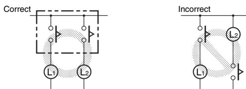
Use the following safety circuit when building a self-holding or self-resetting circuit with the H3Y and an auxiliary relay, such as an MY Relay, in combination.
