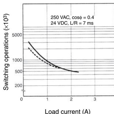
Reference: A maximum current of 0.6 A can be switched at 125 VDC ( $\cos\phi = 1$ ).
