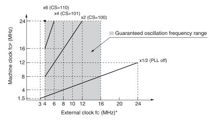
\*: When using a crystal oscillator or a ceramic oscillator, the maximum oscillation clock frequency is 16 MHz.
