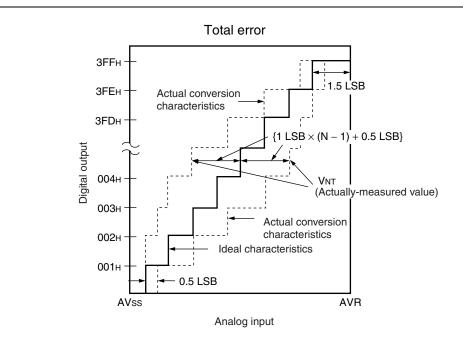
$$Total \ error \ of \ digital \ output \ "N" = \frac{V_{NT} - \{1 \ LSB \times \ (N-1) \ + 0.5 \ LSB\}}{1 \ LSB} \quad [LSB]$$
