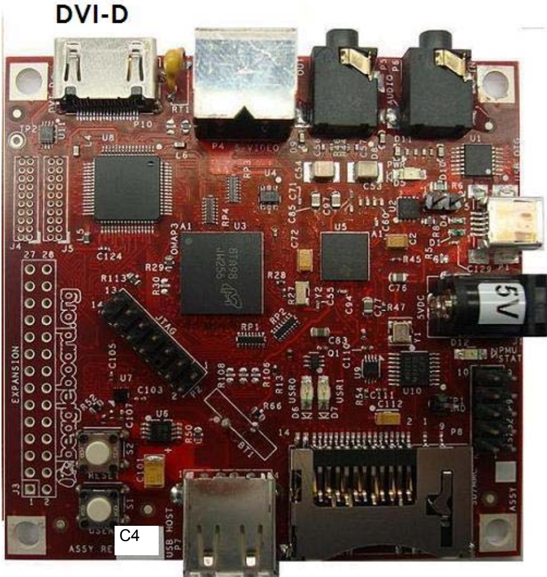
Figure 11. BeagleBoard DVI-D Connection
