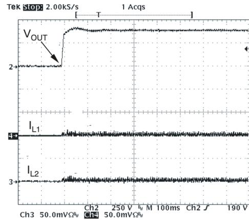
Figure 16. Start-Up at  $V_{IN} = 265 V_{RMS}$ ,
