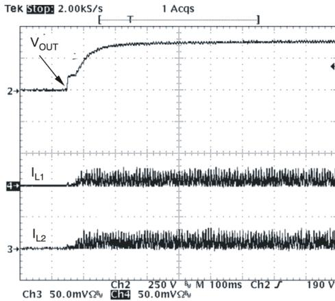
Figure 15. Start-Up at  $V_{IN} = 85 V_{RMS}$ ,
