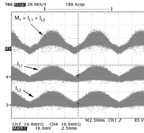
**Figure 14. Inductor and Input Ripple Current at V<sub>IN</sub> = 265 V<sub>RMS</sub>, P<sub>OUT</sub> = 300 W**
