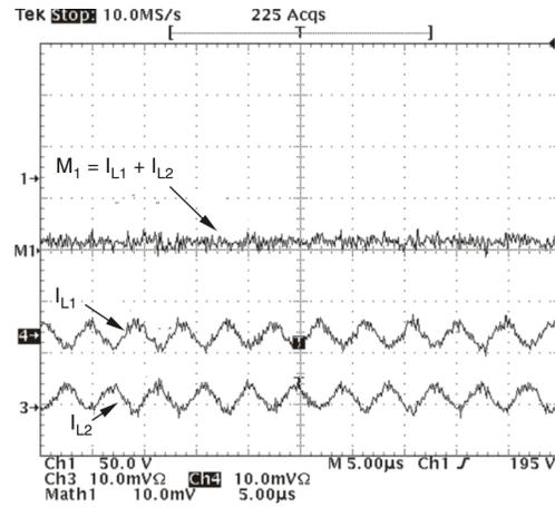
**Figure 12. Inductor and Input Ripple Current at 265 V<sub>RMS</sub> Input at Half Peak Line Voltage**
