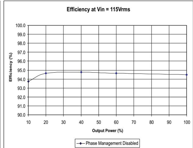
Figure 5. Efficiency at 115 V<sub>RMS</sub>, Without Phase Management
