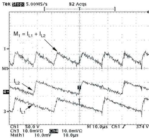
**Figure 11. Inductor and Input Ripple Current at 265 V<sub>RMS</sub> Input at Peak Line Voltage**
