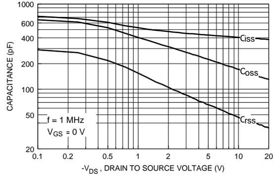
Figure 8. Capacitance Characteristics.
