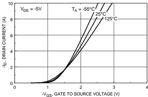
Figure 5. Transfer Characteristics.
