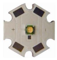
The XLamp XM-L LED is the industry's highest performing, single die white lighting-class LED. The XLamp XM-L is 20% more efficient than the XLamp XP-G at the same current and can deliver 1000 lumens with 100 lumens per Watt efficacy.
