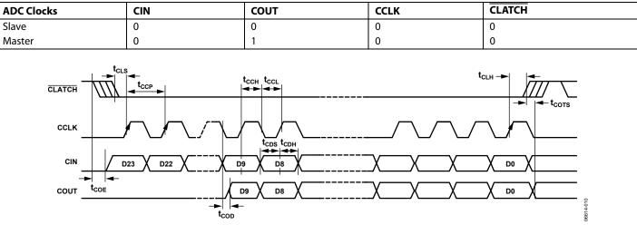
Figure 5. Format of the SPI Signal
