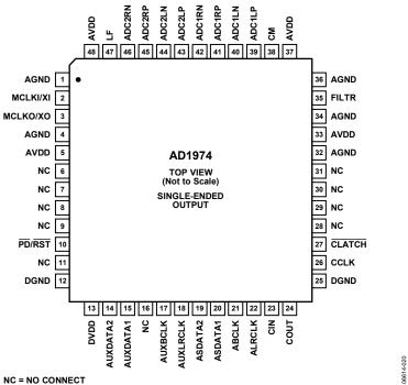
Figure 2. AD1974 Single-Ended Output, 48-Lead LQFP Pin Configuration
