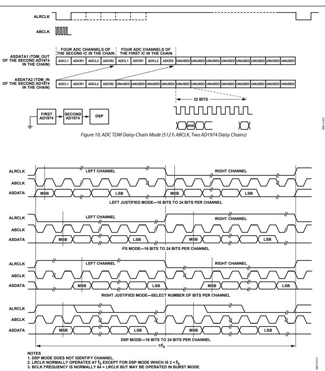
Figure 11. Stereo Serial Modes
