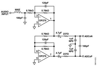
Figure 17. Typical ADC Input Filter Circuit
