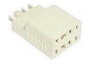
Double adaptor features 6 conductor wiring configuration which suits most telecommunications devices fitted with 605 or 606 telephone plugs Removable panels allow access to change wiring configuration if required. Standard wiring is parallel.
