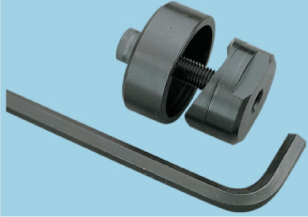
For punching burr-free and accurate holes in sheet metal. Up to 1.625mm thick mild steel, 2mm thick copper, brass and aluminium.
