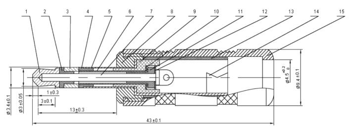
The Terminal Plating Nickel, Thickness 1 µm (Solder)
